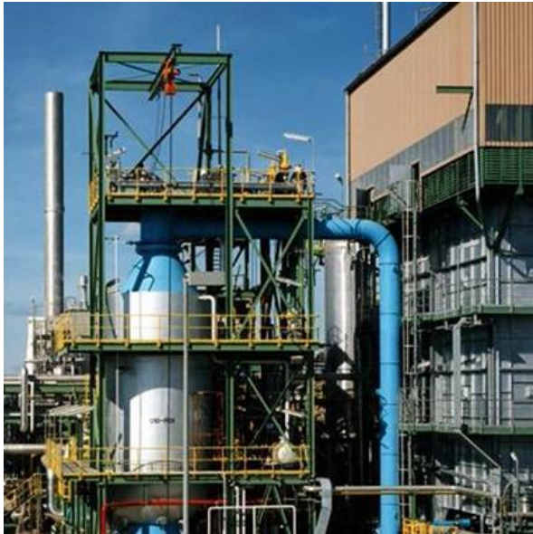
Figure 4: An ATR unit operating in an Air Liquide facility to produce hydrogen gas
